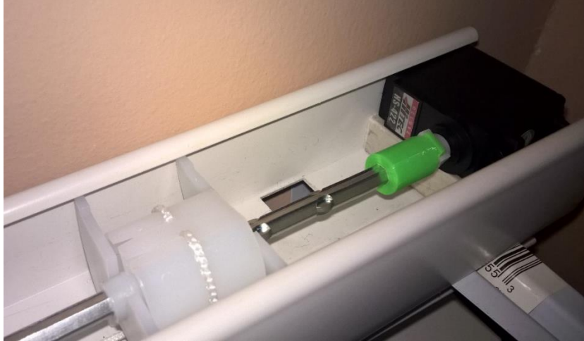
Tilting servo attached to tilting shaft with 3D printed attachment – Fig. 7
