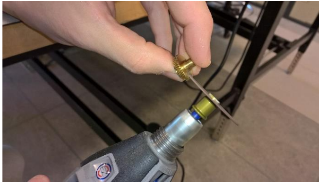
Cutting the limiting pin on lifting servo to allow continuous motion – Fig. 5
