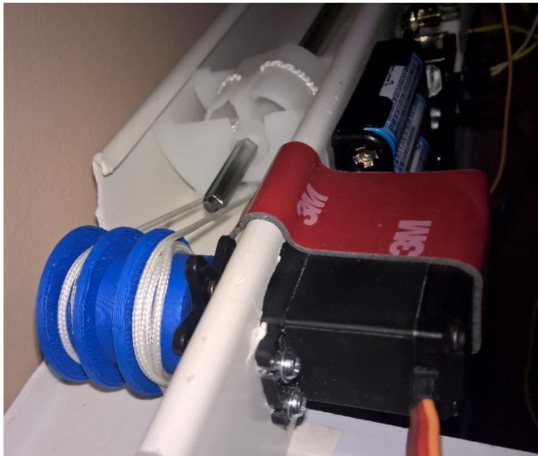
Lifting servo along with the 3D printed spool – Fig. 8
