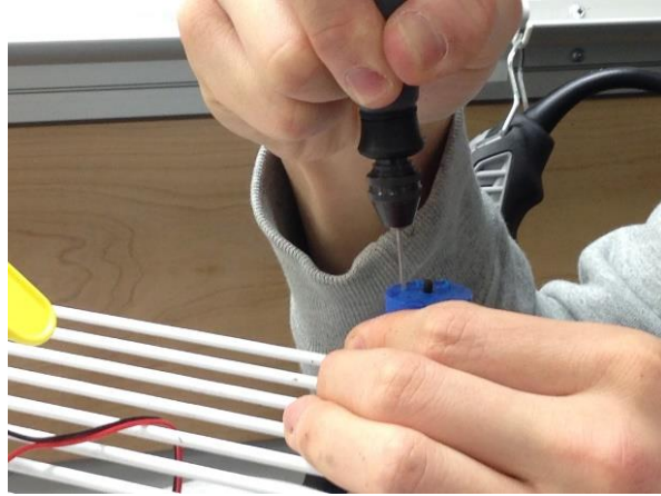
Drilling holes for screws into the lifting servo spool – Fig. 4
